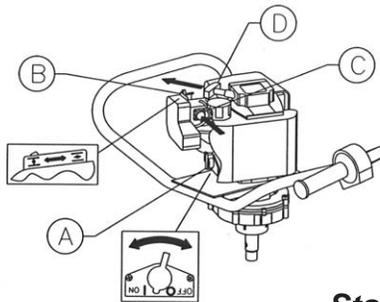
3) Turn the **ignition ON/OFF switch (A)** to the **ON** position.
