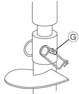
3) Disconnect the spark plug wire. Remove the Hole Digger from the auger. Place the auger back in the hole.
